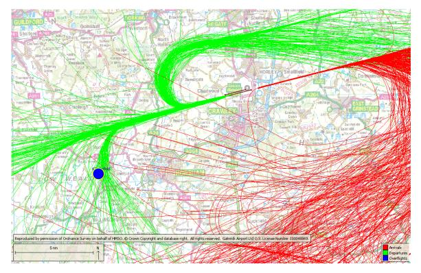
Flight paths for a typical day of departures to the East (Arrivals are shown in Red and Departures in Green). The blue dot shows the location of the noise monitor at Slinfoldl.
